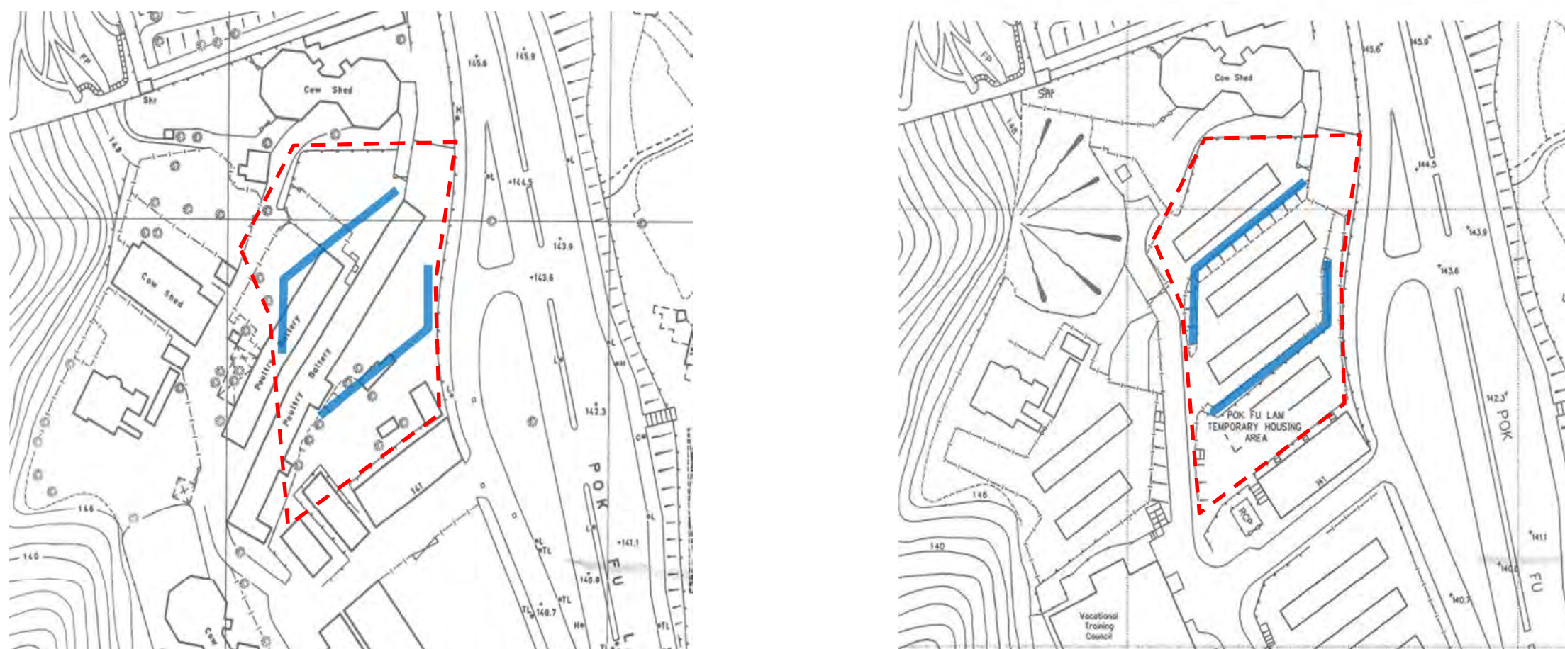
Fig.12 Comparing the layout of the Site in 1983 (left) to 1993 (right). Shade in blue refers to the distinct strata created during the construction of temporary housings in late 1980s, which were not existed in 1983. Dotted line refers to proposed project site. (Source: Survey and Mapping Office, 1983, Ref. no.: 11-SW-17C (Left); Survey and Mapping Office, 1993, Ref. no.: 11-SW-17C (Right); edited by Hebi Chan)
