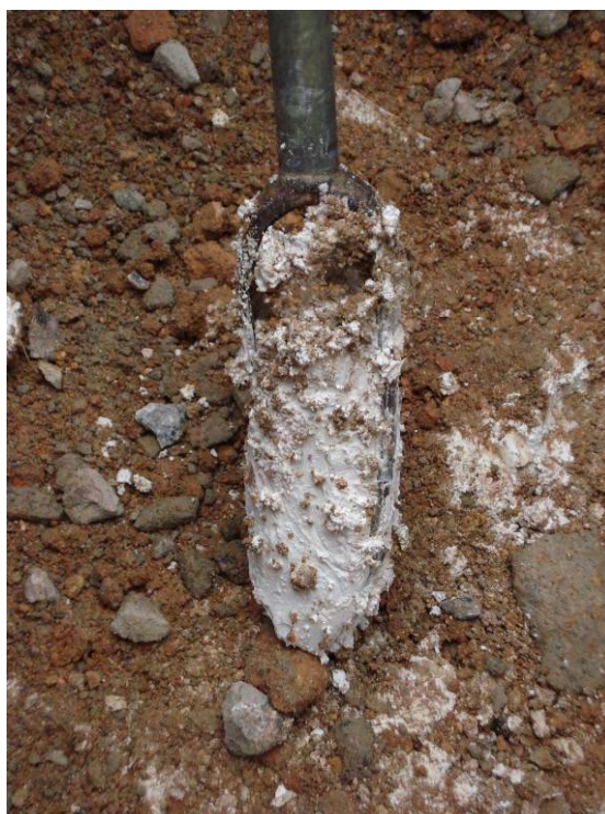
Figure 3.11 White Mortar Drilled by Auger Hole in TTC1
