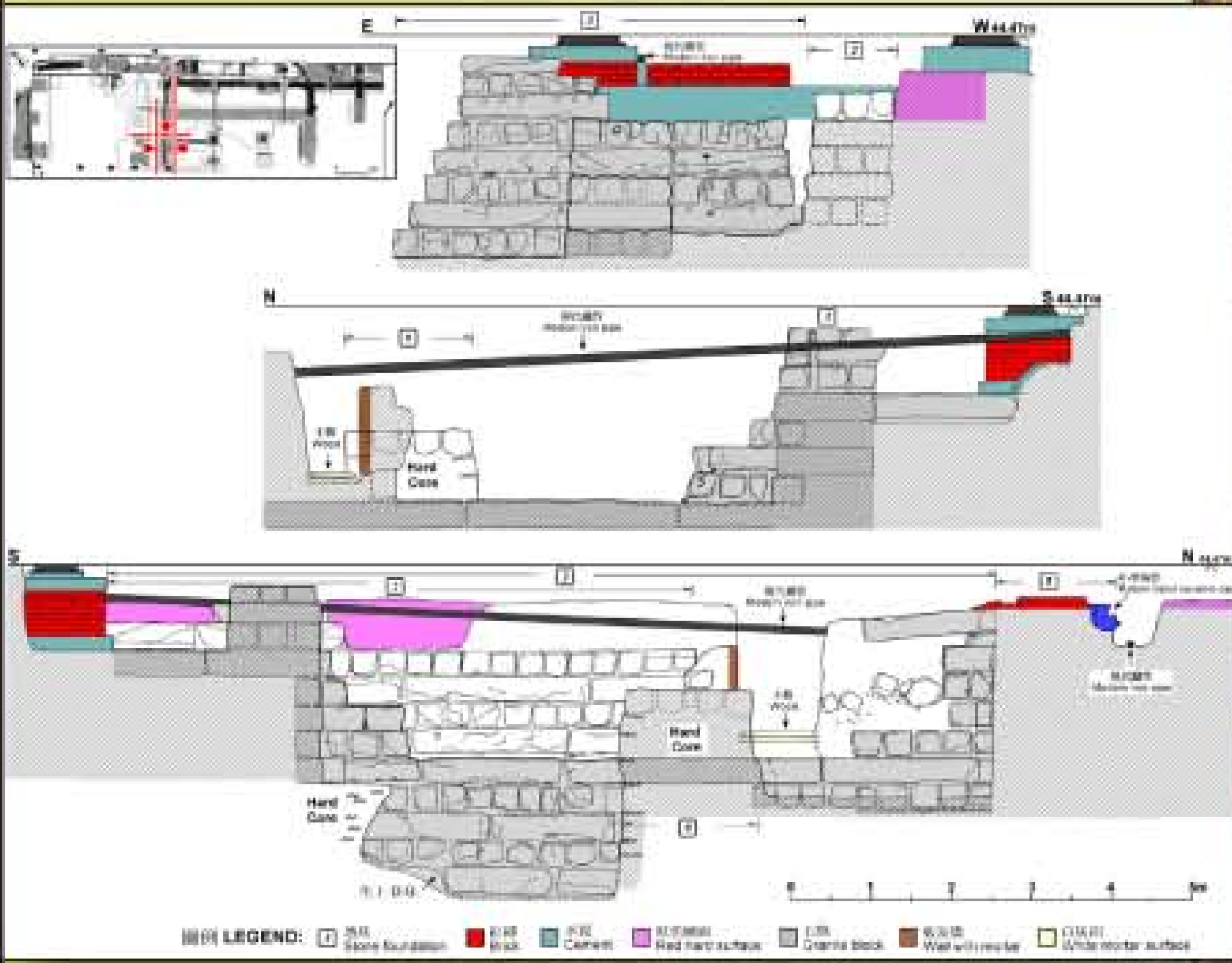
牆基 3 號側視圖 Side Views of Stone Foundation No. 3
