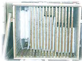
特別為存放彩色玻璃片而設計的密封包裝箱及分隔裝置 The specially designed sealed crate and separation device for storing stained glass panels
