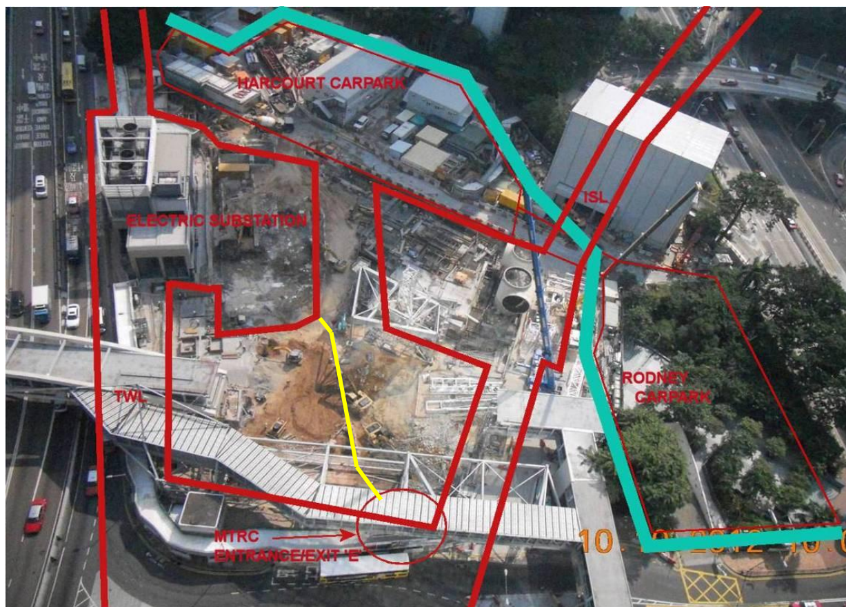
Figure 1b Harcourt Garden and areas of existing impacts marked with thick red line (MTR Corporation's Island Line and Tsuen Wan Line and the Electric substation), thin red line (underground carparks) and aqua blue line marks the cooling mains for the shopping malls in the vicinity. The seawall fragment is marked in yellow. Please note that in addition to the marked impacts archaeological evidence shows that Harcourt Garden surface level was cut down to a maximum of 4mPD. Current view shows the area around the seawall at around 2.5mPD.
