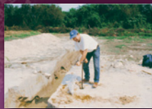
利用鑽探工具採集土壤樣本 Collecting soil samples by the hand auger
